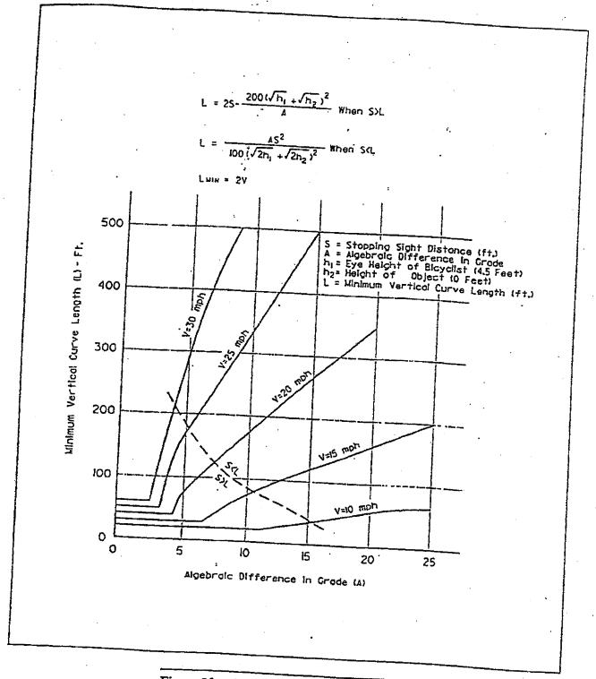
Figure 10. Minimum Length of Vertical Curves.
